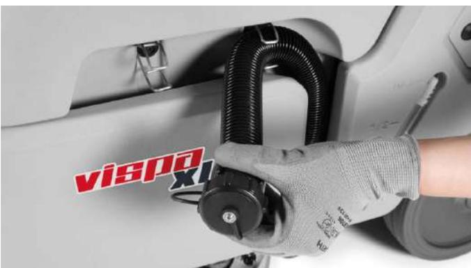
Full access to components makes it easier to carry out both routine and extraordinary maintenance. The recovery tank has a handle so it is easier to lift and empty. To further facilitate this operation, the Vispa XL dirty water tank can also be emptied through the pipe on the side of the machine.
