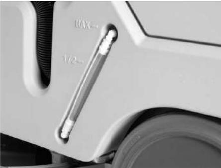
The solution level in the scrubbing machine is always visible, thanks to the transparent indicator on the side of Vispa XL.
